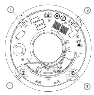
Check that each of the 4 swing out clamps are rotated inwards. Push the loudspeaker through the mounting hole and position flush with the ceiling. Whilst holding the loudspeaker in place tighten each of the mounting screws using a No. 2 Pozidriv® screw driver in the order shown in the diagram (left). When an increase in resistance is felt the clamp is in position.
